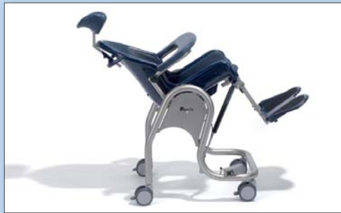
Tilt-in-space seat angle is steplessly adjustable via a gas pressure spring from (-) 5° to 30°
