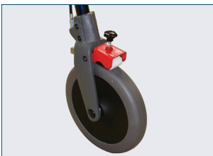
Slow down brakes mount on rear wheels. They are independent of the braking system. A nylon wheel rides on the tire to add tension to slow the walker. Knob on top adjusts the tension on each side.
