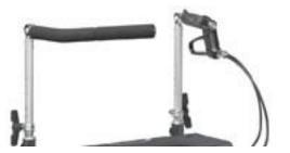
HP handles or hemiplegic handles are mounted on the Symphony model. The one hand braking system uses a padded bar on the non-braking side. This bar can be adjusted in height and angle to the body, so that you can push with your body while steering and braking from the other side.
