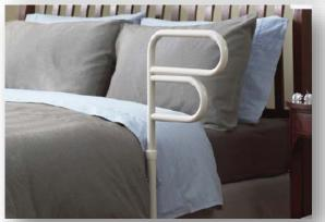
**70000 Arcorail®** is a rotating, professional-grade bedside handrail, which provides maximum bedside mobility for home, clinical care, and hospital settings. Patented rail rotates 360° and locks in place every 90°; totaling four locked positions. Vertical floor tube has multiple height adjustments, 23"-33" and fits all bed sizes. Second loop can be removed for taller mattresses up to 24" high. Arcorail® s surface is treated with an anti-bacterial powder coating.
