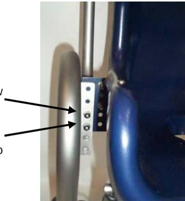
Now adjust the gas pressure spring (below) so that the seat angle is correctly set again. To do this, unscrew the screw of the gas pressure spring holder <arrow> completely out of the threaded plate and replace it at the correct height.
